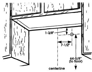
To wire through rear, mark a line 7-1/2" from the right of the centerline on the wall. Mark the point on this line that is 64-5/8" from the floor (or 1-3/8" from underside of cabinet). Drill a 1-1/4" diameter hole through wall at this point.
